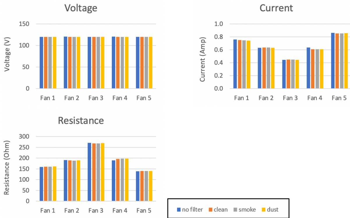
FIGURE 8. VOLTAGE, CURRENT, AND CALCULATED RESISTANCE LISTED FOR NO FILTER, CLEAN FILTER, SMOKE LADEN FILTER, DUST LADEN FILTER CONDITIONS FOR THE FIVE FANS. FAN 1 DATA IS THE AVERAGE OF FAN 1-1 AND FAN 1-2.
